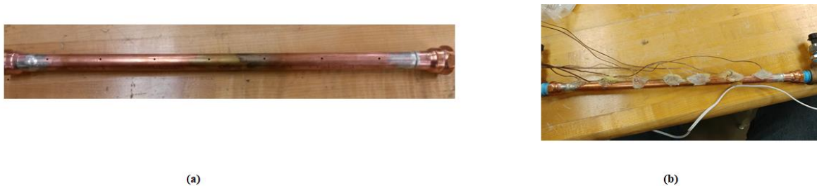
Figure 4. (a) Copper tube with holes and (b) thermocouples embedded and glued into the pipe
