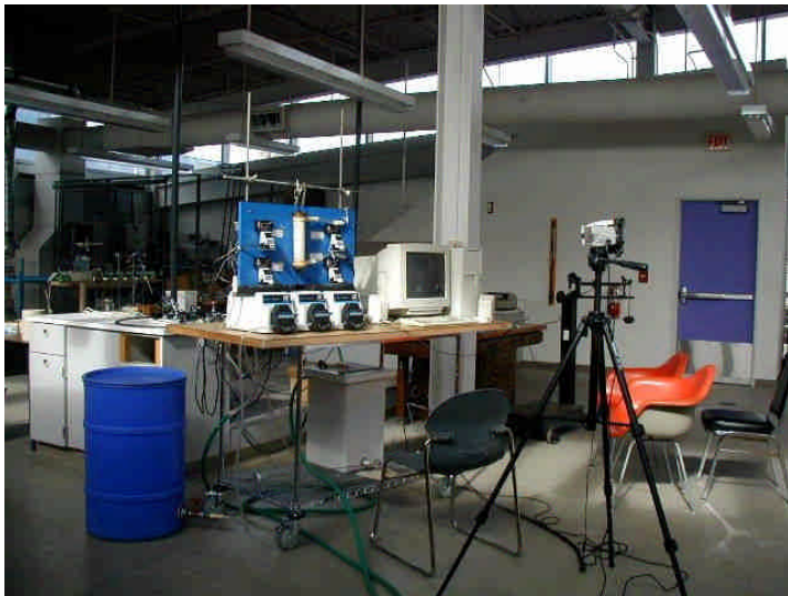
Figure 2. Photograph of dialysis experiment. The module is the white cylinder in the middle of the blue board. The blue cylindrical tank to the left contains the salt solution feed.
