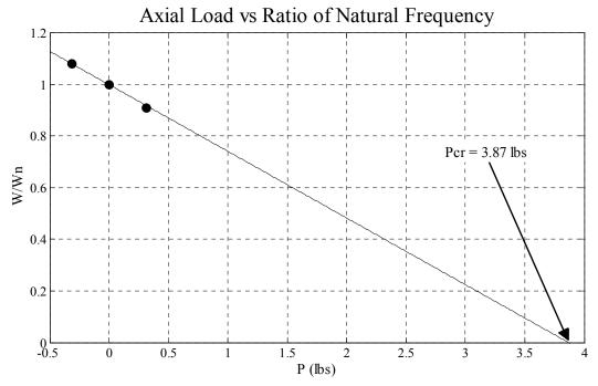
Figure 5: Experimental Results, Axial Load (P) vs. Natural Frequency (w<sup>2</sup>/w<sub>n</sub><sup>2</sup>)
