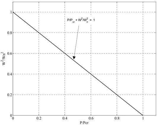
Ratio of Natural Frequency With Respect to Critical Buckling Load
