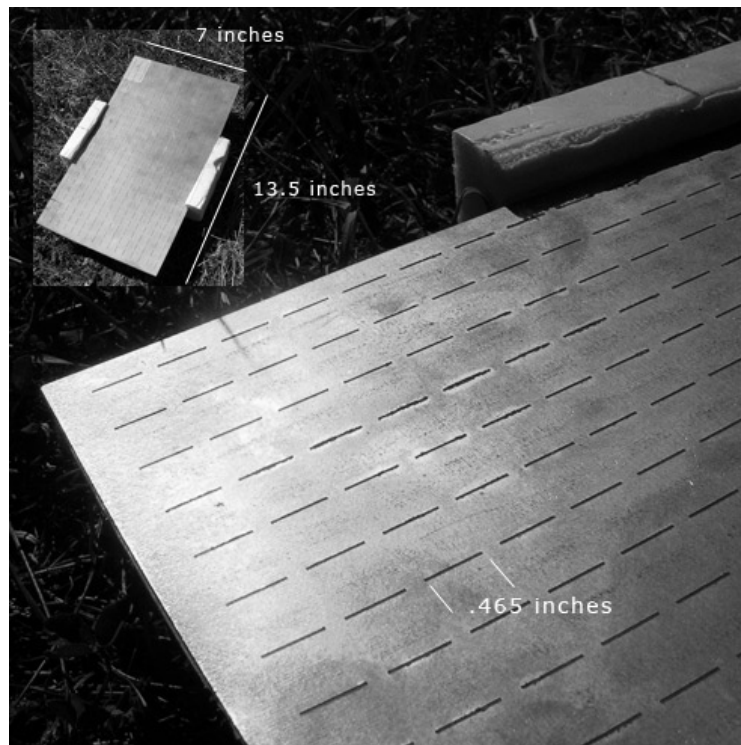
Figure 4 - Frequency Selective Surface - the individual slots measure 0.465 inches, corresponding to the half-wavelength resonant frequency after taking into account the dielectric material of the supporting substrate.
