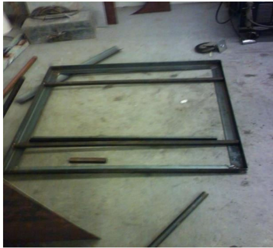
Fig. 5: Base frame to hold the machine and to attach the lifting devices
