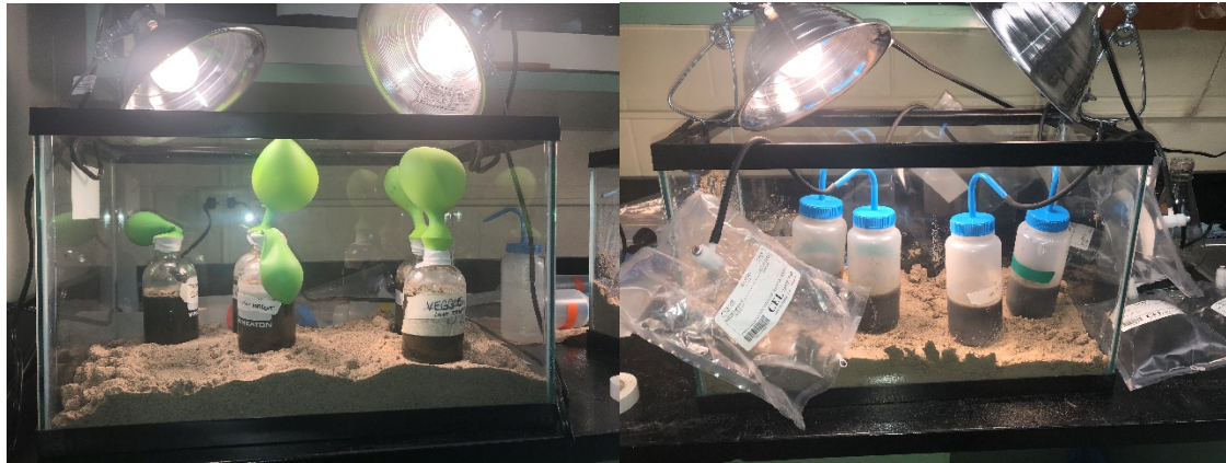
Figure 4. Anaerobic digestion bottle reactors using balloons (l) and Tedlar bags (r) to collect biogas
