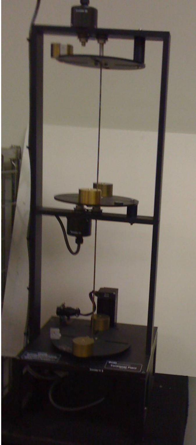
Figure 2: ecp Model 205 rotational mass-spring-dashpot apparatus for evaluating one, two, or three DOF systems: forced or unforced.
