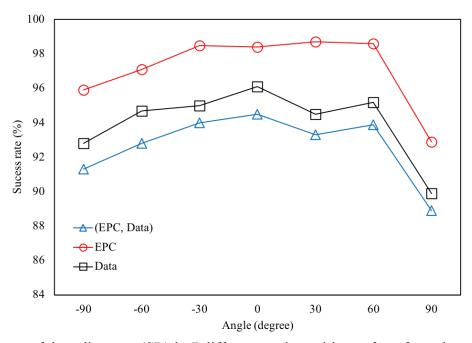
Figure 4. Successful reading rate (SR) in 7 different angle positions of tag from the reader where  $A_T = \{-90^\circ, -60^\circ, -30^\circ, 0^\circ, 30^\circ, 60^\circ, 90^\circ\}.$
