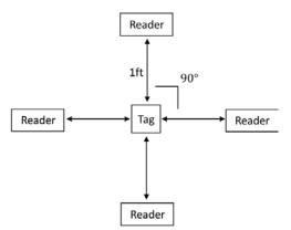
(c) Experimental setup for various position of reader in angle,  $A_R = \{0, 90, 180, 270^\circ\}$
