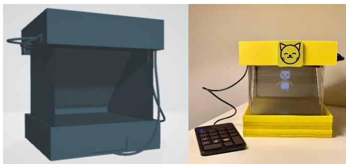
Figure 1: CAD Drawing and Final Build of the “PepperPet” Case
