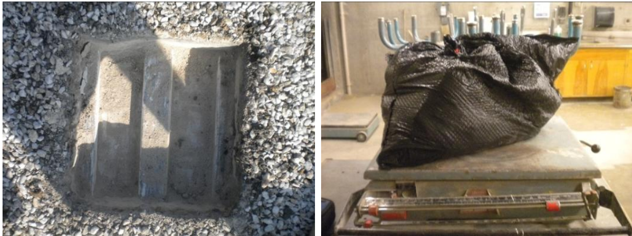
Figure 8. Bridge House Roof Weight Verification 9
