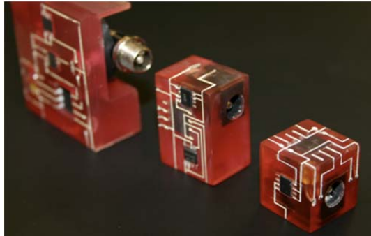
Figure 1. Miniaturized 3D electronics fabricated using LM technologies: evolution of a 3D magnetic flux sensor illustrating increased levels of 3D component placement and conductor routing, leading to improved integration and packing.
