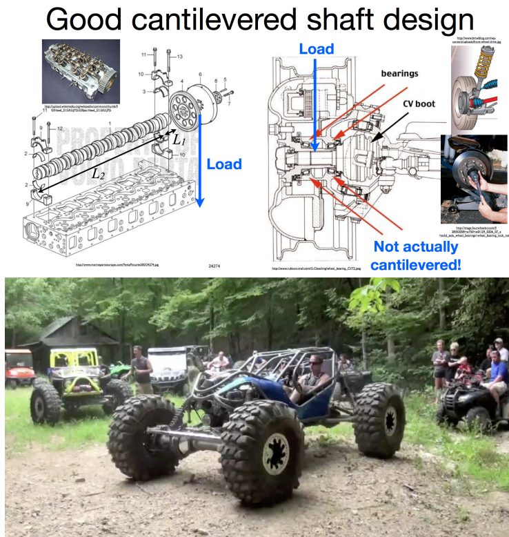
Figure 3: Examples of well-supported shafts with various forms of constraint and coupling. Video of off-road vehicle is available at [5].
