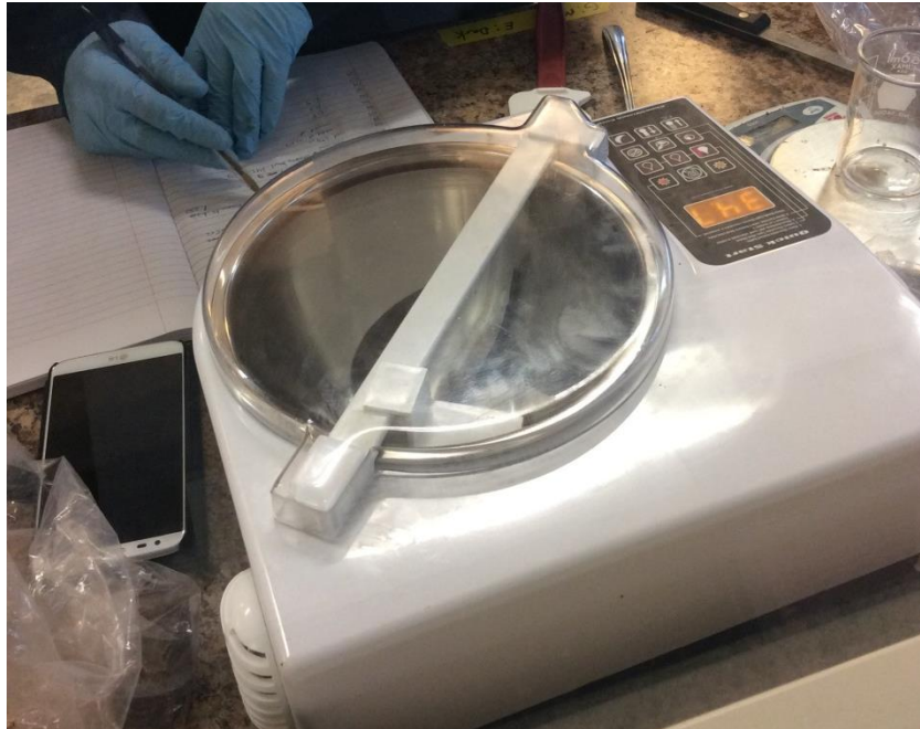
Figure 1. A student using a tempering machine to temper milk chocolate, as introduced in the fourth experiment. The tempering machine is used to automatically control the melting of chocolate to select for the beta crystals, which possess the highest melting point and produce the desired characteristics for enrobing chocolate. The machine pictured is a ChocoVision ® C116MINIREV1, which is roughly 360 USD at retail.
