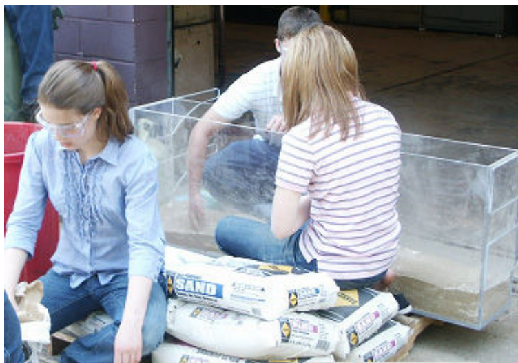
Figure 2. Preparation of simulated lunar regolith with free iron, with simulant tank pictured.
