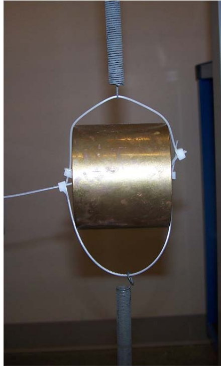
Figure 5. A mass with a secondary spring that is used to introduce students to multiple degree of freedom systems.
