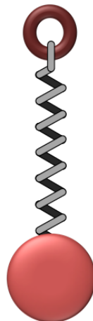
Figure 2. Spring/mass system used in vibrations course to introduce the concept of stiffness and mass and its relationship to the natural frequency.
