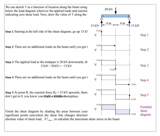
The method for drawing a shear diagram is shown below in 6 diagrams. Accompanying text and equations are aligned with each diagram. Each image builds on the previous frame, until the shear diagram is complete.
