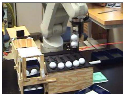
Innovative end-effector design to pick up multiple balls at once
