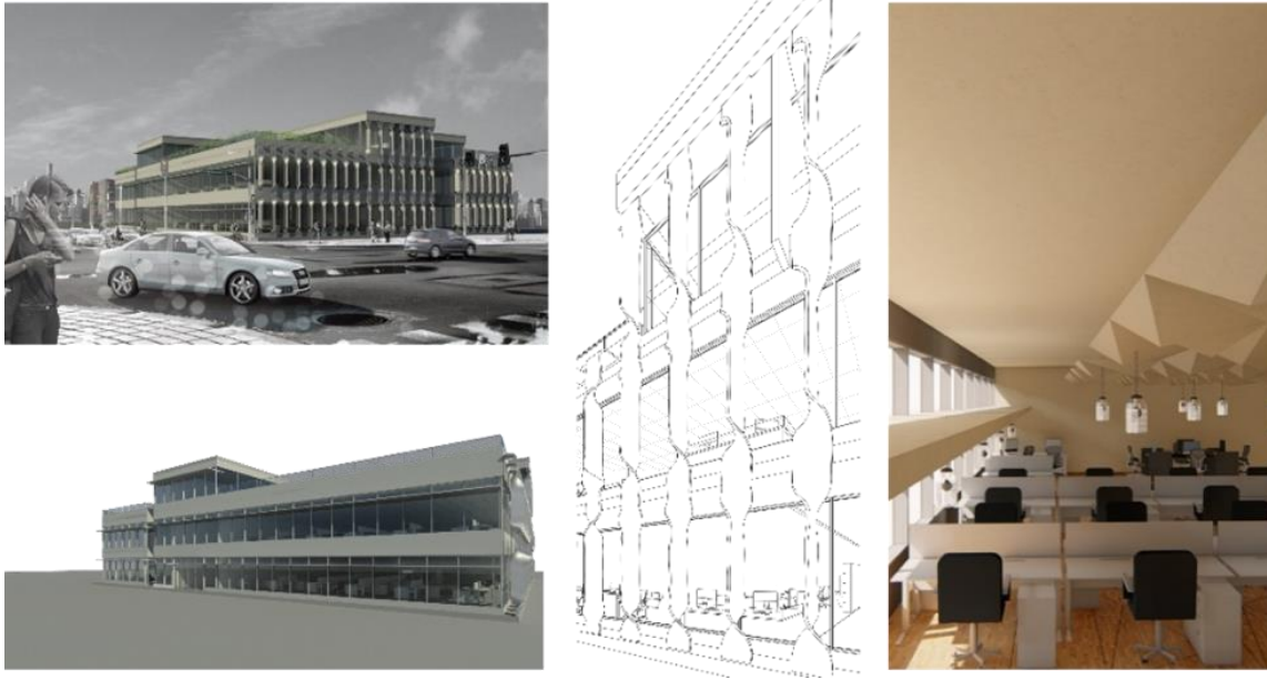
Figure 12: Shading devices design, vertical fins on the east (top left), horizontal overhangs on the south (bottom left), vertical fins technical drawing (middle), overhangs extend to a light shelf inside the space (right)
