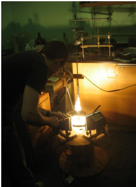
Fig. 3 a) Student working in the lab on crystal synthesis by means of electro spray; b) the high voltage module.
