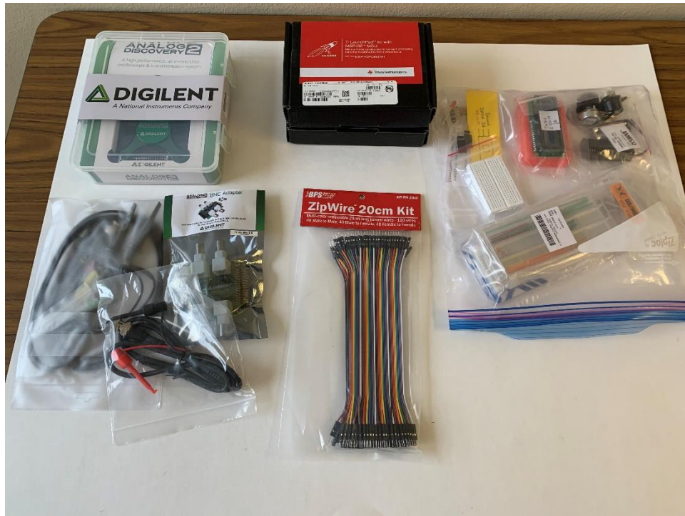
Figure 2. Microcontroller Lab Kit: Digilent Oscilloscope/Logic Analyzer, TI Microcontroller LaunchPad (x2), accessory parts
