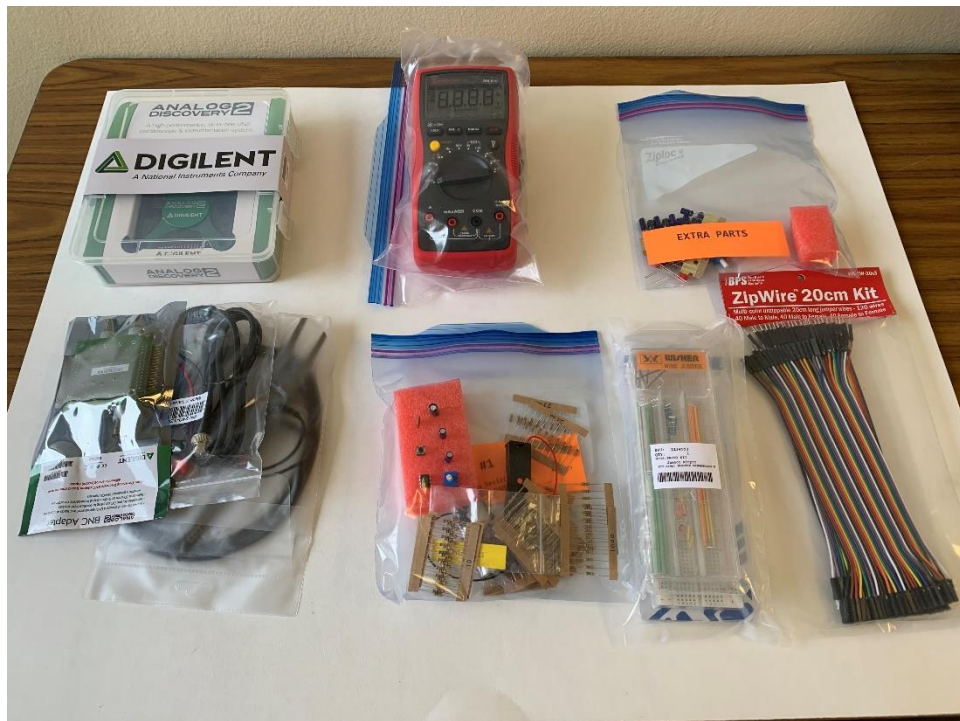
Figure 3. Electric Circuits Analysis Lab Kit: Digilent Oscilloscope/Logic Analyzer, Volt-Ohm meter, accessory parts
