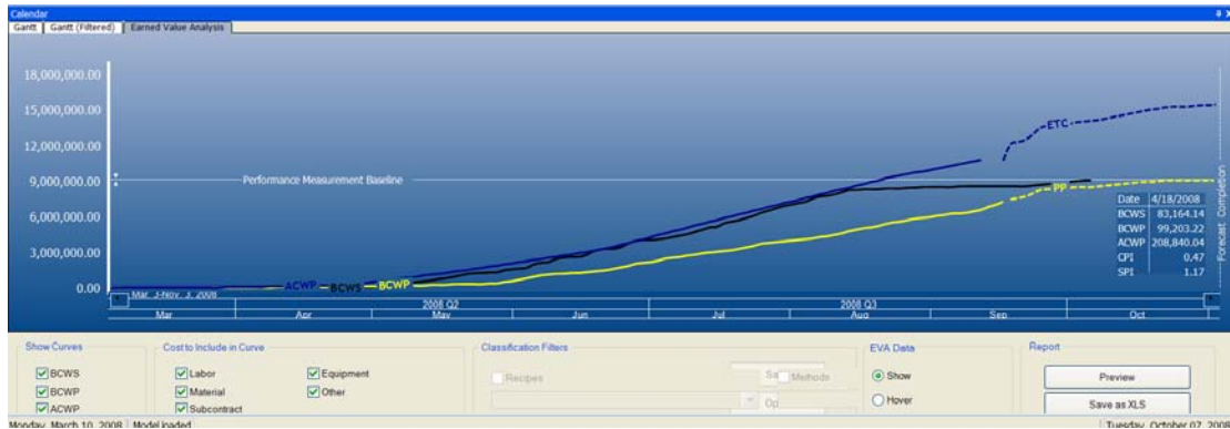
Figure 13. Cash Flow Analysis in Vico 5D Presenter (picture courtesy of Vico Software)
