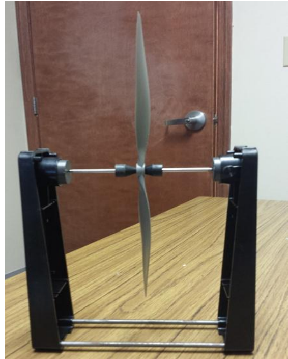
Figure 6: The propeller balancer with a propeller mounted. The metal rod that holds the propeller is suspended by magnet on
