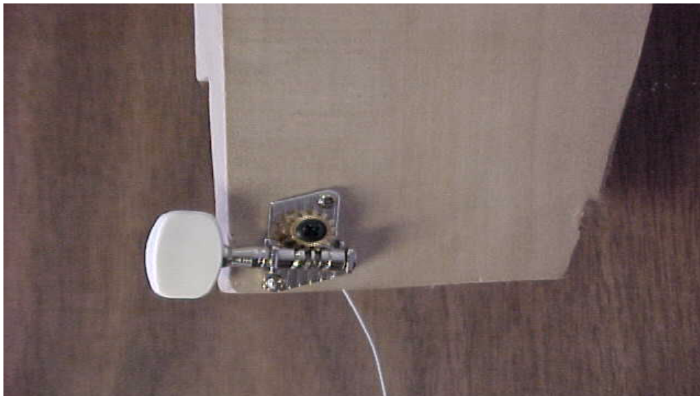
Figure 5. Guitar Tuner: Example of a Worm Gear.
