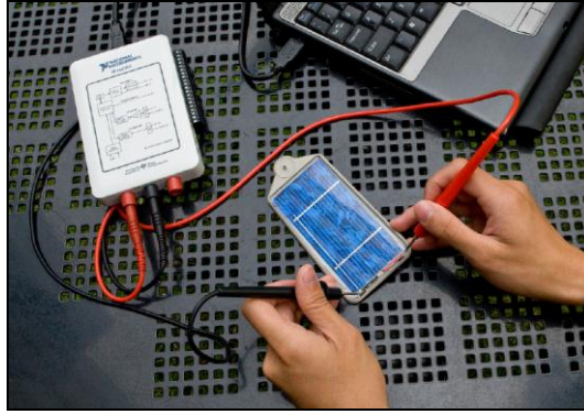
Figure 1:NI myDAQ being used to probe the output of a Solar Cell
