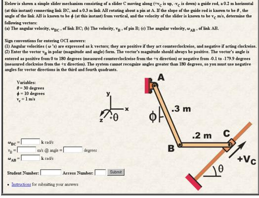
Figure 3: Four Bar Slider Problem, Rigid Body Kinematics
