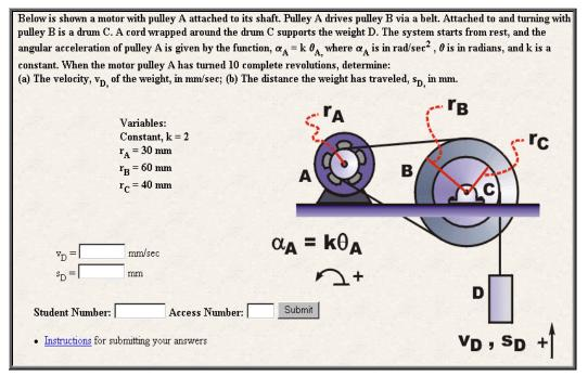
Figure 4: Fixed Axis Rotation Problem, Rigid Body Kinematics
