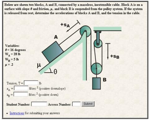
Figure 5: Two Blocks Problem, Particle Equations of Motion
