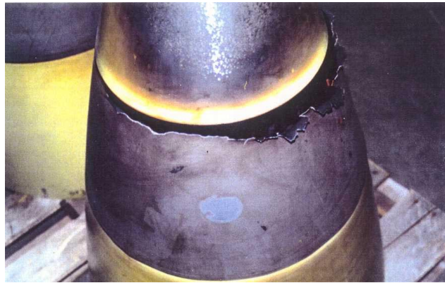
Figure 5. Antenna Failure for EDP3
