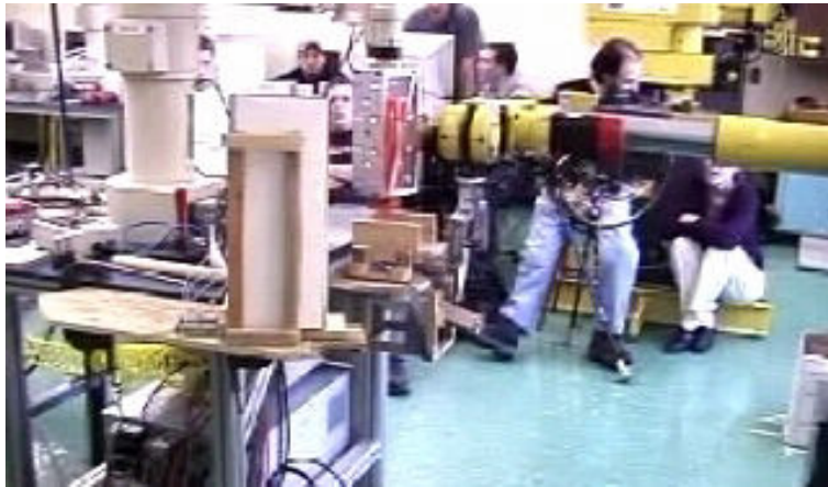
Figure 2 A Cylindrical Robot working with a SCARA Robot to simulate a machine loading and milling operation
