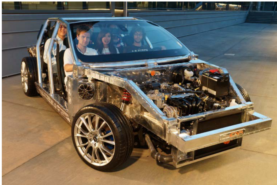
Figure 17. Final NBT Concept Vehicle with 6 Seated Occupants
