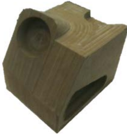
Figure 16. Wooden Block for A-Pillar BIW Space Frame Nodal Joint
