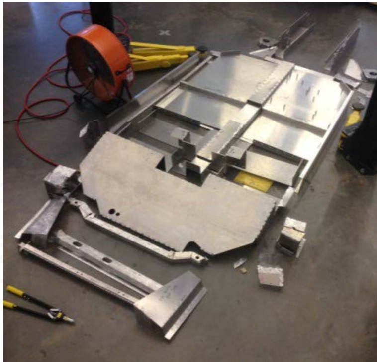
Figure 15. Final Test Assembly of Folded BIW Components
