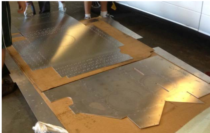
Figure 13. BIW Structural Components before Folding
