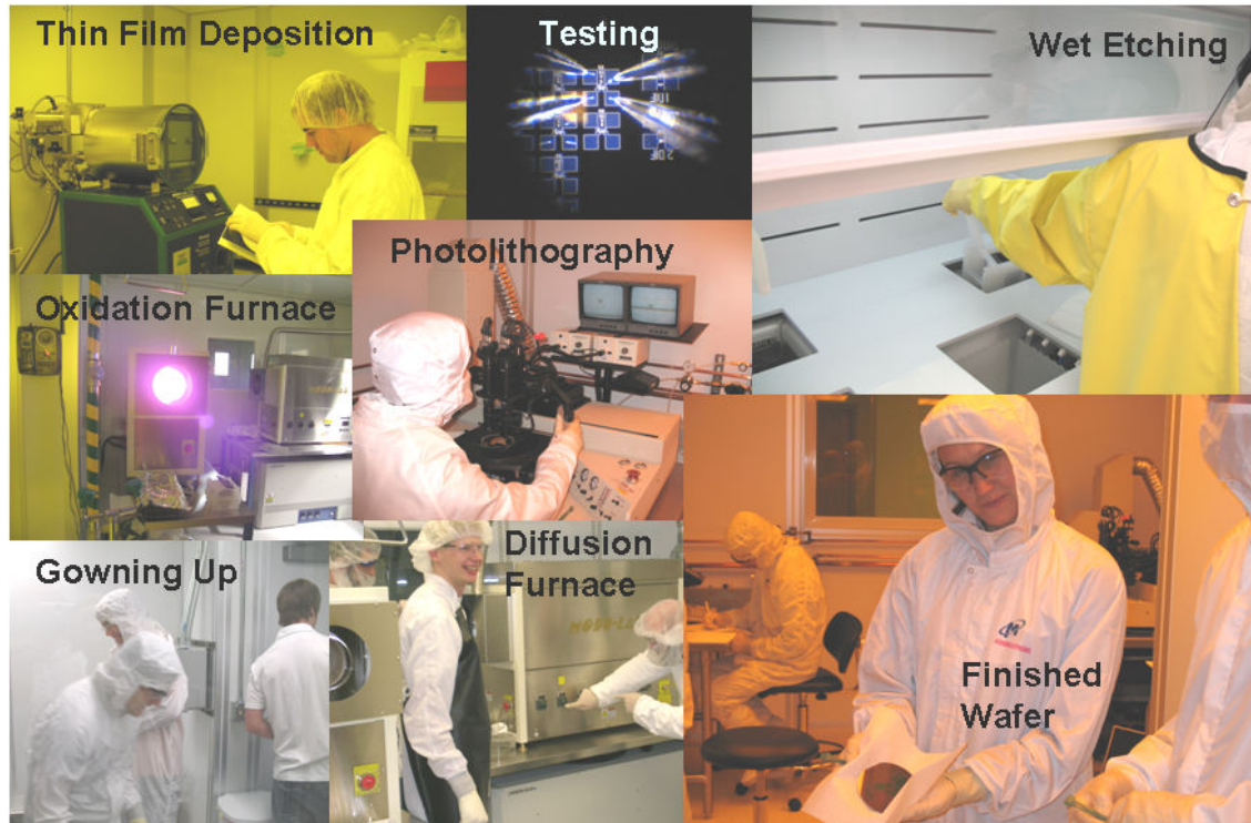
Figure 2. Students going through the steps of the flowchart Lower Left: Student gowning up to go into the clean room Middle Left: The oxidation furnace used to produce a conformal silicon oxide coating covering the wafer Upper Left: Evaporation System for metal deposition Upper Middle: Image of a device being tested Center: Student performing photolithography with the mask aligner Lower Middle: Student setting the temperature on the diffusion furnace Upper Right: Student etching the silicon dioxide from the silicon wafer Lower Right: Student showing the completed wafer
