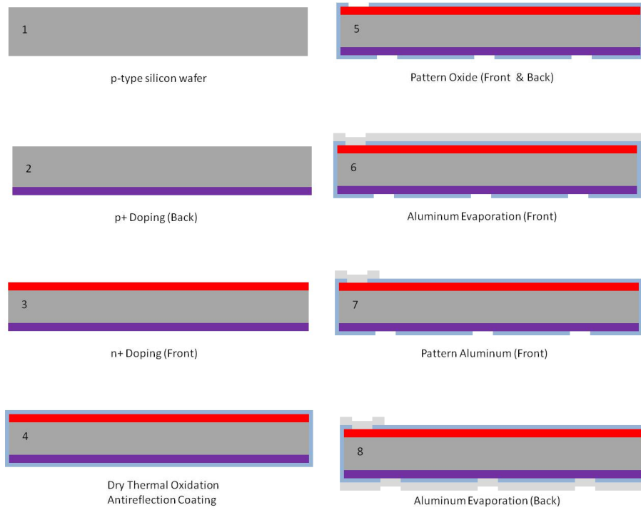
Figure 3. The fabrication sequence to produce a silicon solar cell.
