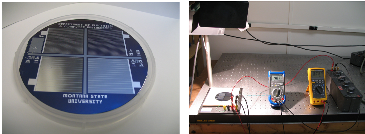
Figure 4. The fabricated wafer with 4 solar cells and the characterization set-up.
