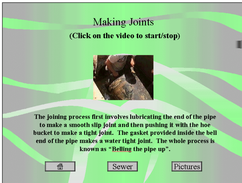
Figure 5. Video of making sewer pipe joints
