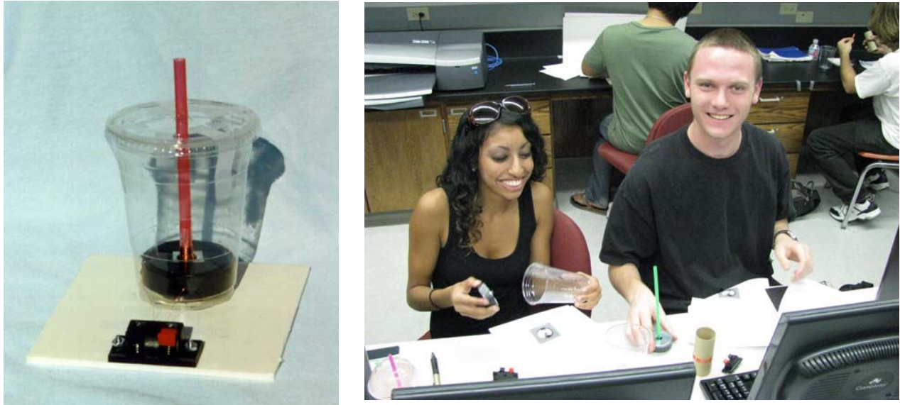
Figure 2: Simple Speaker Made From a Plastic Cup That Requires Limited Work Space.
