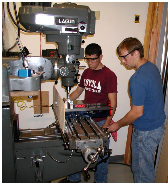
Figure 6: A student team machining the cylinder for their air-engine.
