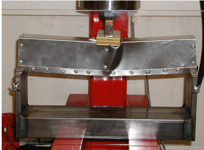
Figure 4: Sample rectangular cross-section beam in test fixture, after failure.
