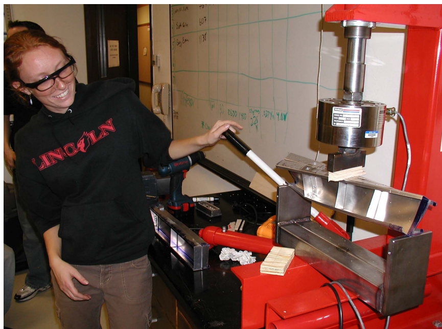
Figure 5: Sample I-beam in test fixture, exhibiting lateral torsional buckling.
