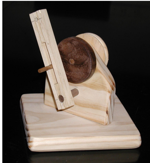
Figure 1: Sample fast-return actuator -- the students' first woodworking project. Pulley at rear is for optional drive system by DC motor and pulley.
