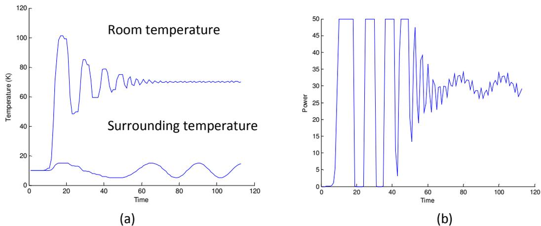
Figure 5 The room temperature and the surrounding temperature (a) vs. time.
