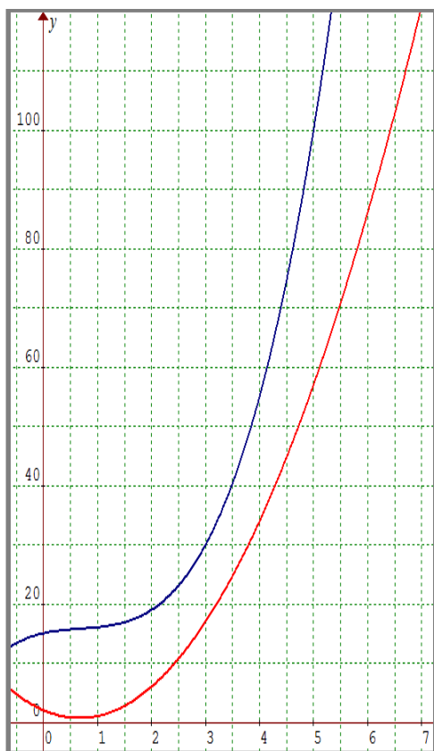
Fig. 6. The water level in a tank is modeled with a cubic function (blue graph) and its derivative is a quadratic function, a parabola (red graph).
