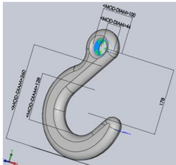
Figure 4 Solid model of the hook and a constraint being applied at the hole
