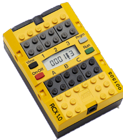
Figure 1. The RCX has three ports (1,2,3) that can take input from sensors and three ports (A,B,C) that can output power to motors, lights, or sound makers. It runs on 6 AA batteries and can hold up to 5 different programs: each executing up to 10 simultaneous tasks. Programs are downloaded to the RCX via an IR tower connected to a computer's serial port.
