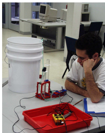
Figure 16. Students used the RCX to start and stop the water flow and log the time it took for the Styrofoam wedge to cross in front of the light sensor and measured the amount of water in the graduated cylinder.
