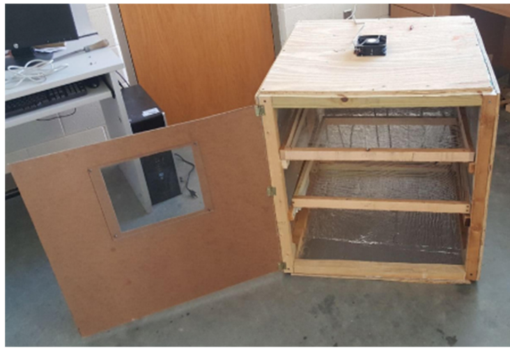
Figure 7 the Assembled Dryer Prototype
