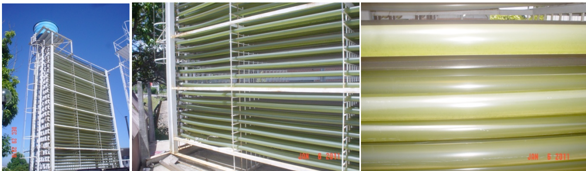
Figure 1. Microalgae growth in compact photobioreactor (5 m × 2 m × 8 m) at the Brazilian university
