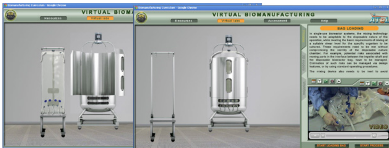
Figure 3. Loading a disposable bag into a bioreactor. An example of an assembly exercise for a virtual single-use bioreactor. Instructions for loading a disposable bag are displayed in the top right panel. A video presenting preparation of a disposable bag is shown in the bottom right panel.
