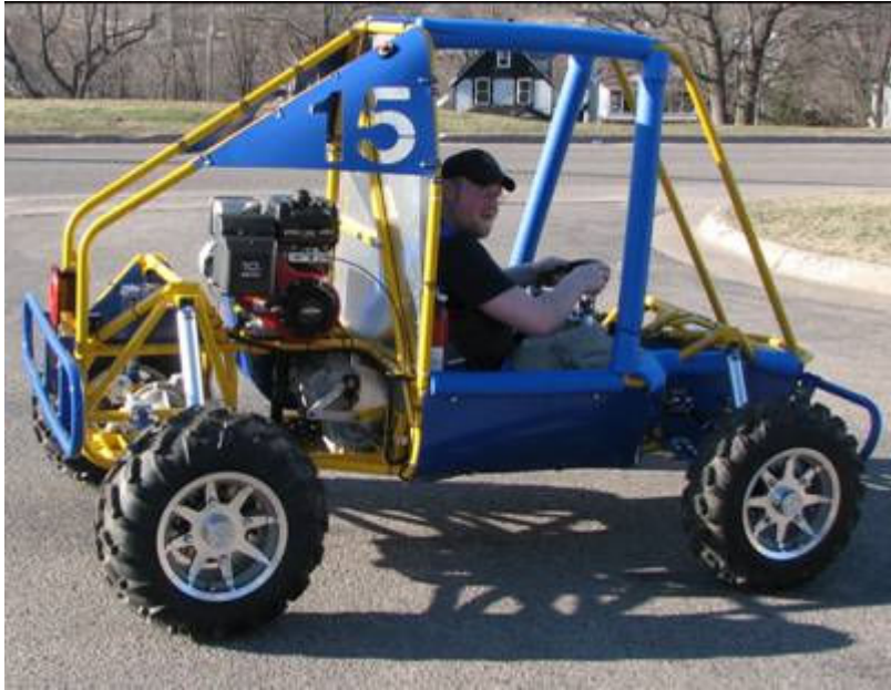
Figure 4: A photo of the previous year Mini Baja vehicle showing the frame rear part and the power train
