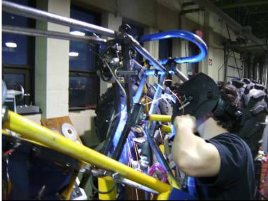
Figure 7: Welding the frame
