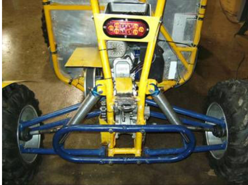
Figure 9: The new rear part of the vehicle with the suspension, power train, and new frame.
