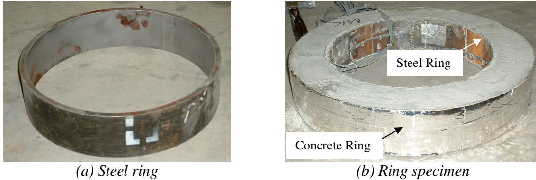
Figure 2. Restrained ring specimen.
