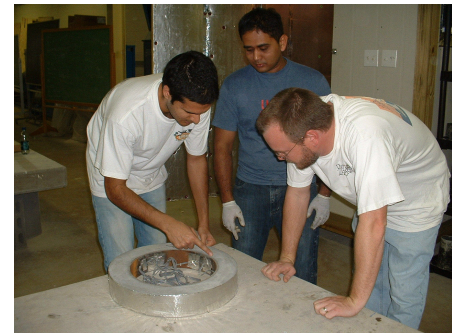
(c) Simulation of restrained shrinkage
