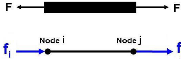
Figure 1 Comparison of an axially loaded bar and a 1-D Bar element
