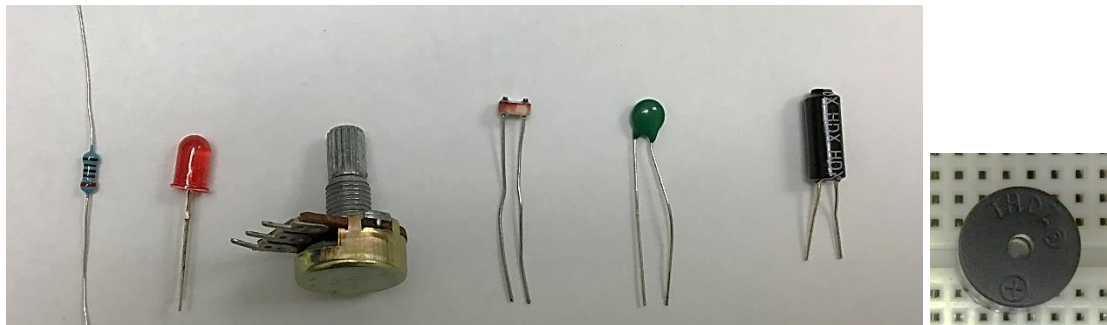
Figure 1: From left to right - Resistor, LED, Potentiometer, Photocell (Light Sensor), Temperature Sensor, Tilt Switch, and Piezo Buzzer
