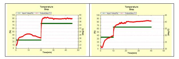
Samples of the tuning tests run by students are shown below. The one on the left is a "good" test; it has fast response and no overshoot. The one on the left with its output oscillation and large controller action would likely be considered a poorly tuned controller.
