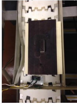
Figure 12. A part on conveyor to be identified by the vision system
