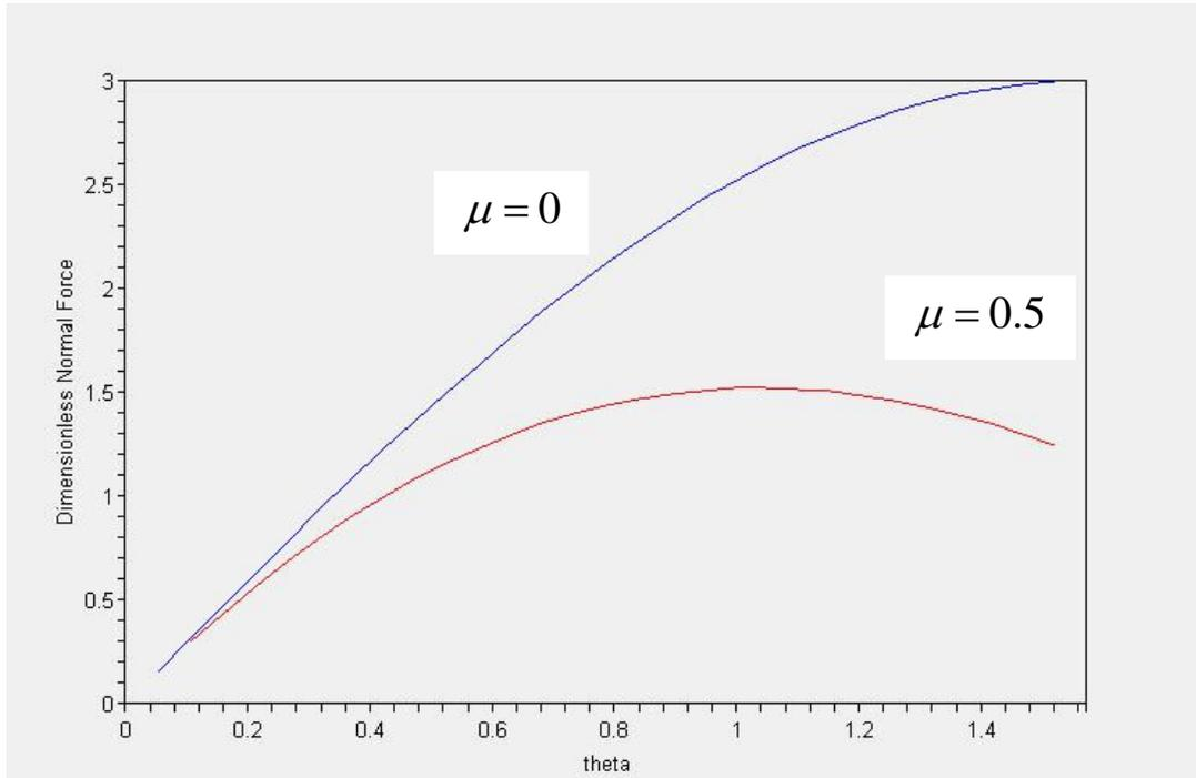
**FIGURE 10 – NON-DIMENSIONAL NORMAL FORCE VERSUS  $\theta$ ,  $0 \leq \theta \leq \pi/2$**
