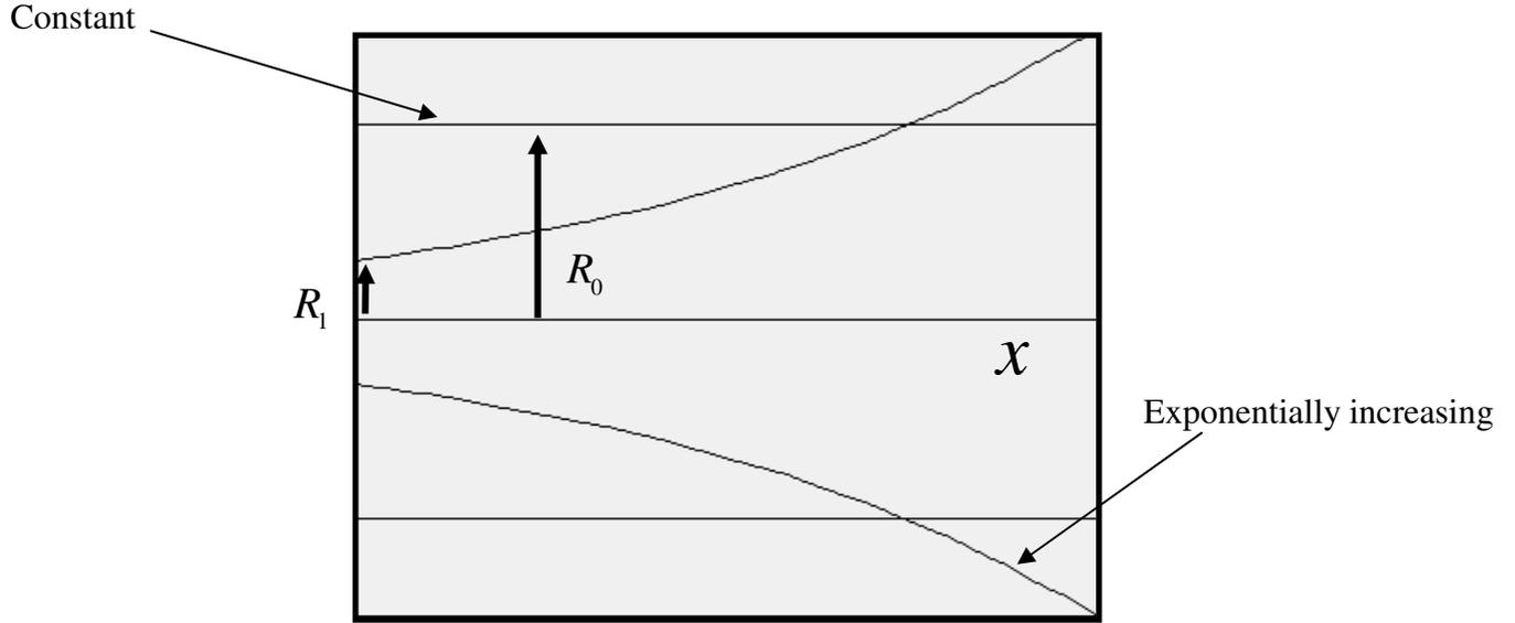
FIGURE 4 –CONSTANT AND EXPONENTIALLY VARYING SHAFTS
