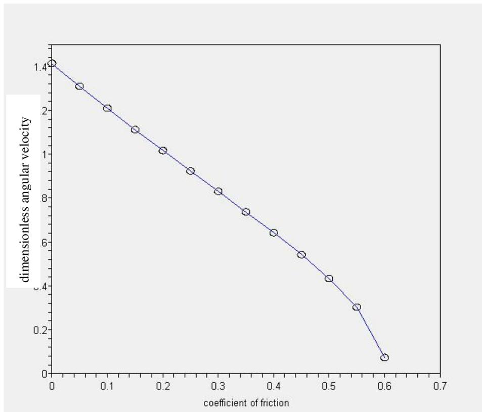
**FIGURE 9 – COEFFICIENT OF FRICTION VERSUS ANGULAR VELOCITY AT  $\theta = \frac{\pi}{2}$**
