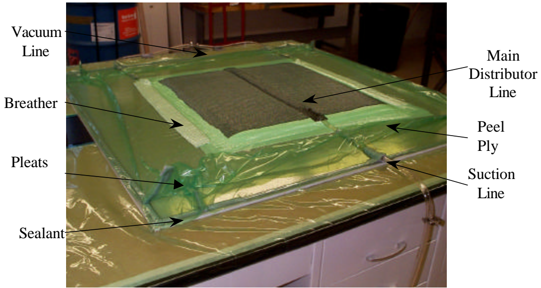
Figure 1 VARIM fabrication setup photograph
