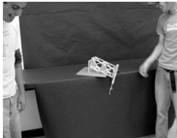
Loading = 4.0 lb = Collapse
