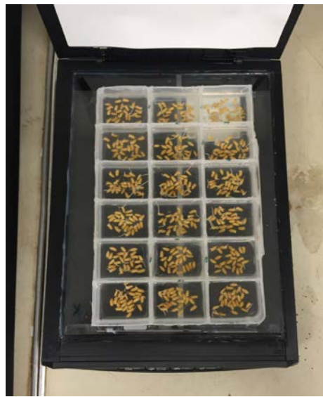
Figure 4: Scanning bed with seed organizer during experiment.
