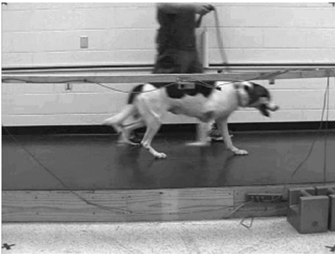
Figure 4. Measurements of canine stride length were made using the prototype video system.
